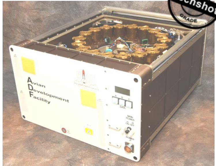
The Avian Development Facility is shown with its top covers removed, revealing its upper carousel and 18 sample containers (non-standard Velcro® was attached during the STS-108 mission).
