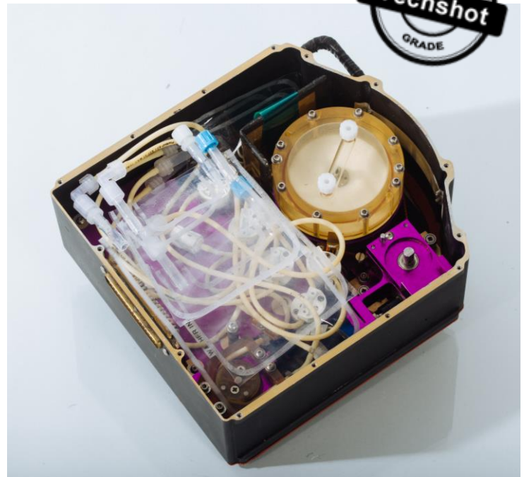
CELLCULT cassette is shown without top cover. A gasket around the outer edge provides one of the two levels of safety containment.
