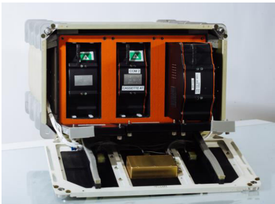
Fluid Processing Cassettes are operated inside the Techshot ADvanced Space Experiment Processor.
